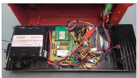
a remote charging jack. There is also a Phoenix toggle switch for volume control. These need to be accessible by the operator. After careful measurement and inspection, it looks like the on/off switch and charge jack can be mounted on the front of the tender, but no room for the volume there. So the volume switch will be floor mount-
