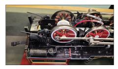
through the hole, into the motor cavity, and to the motor wires. Each side of the cable is loosely covered with black heat shrink to hide the red wire. The cable and motor wires are soldered together and covered with heat shrink tubing. Polarity doesn't matter, as we can easily fix that in the tender.
