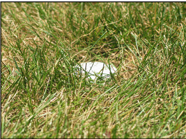
When not in use, the mounting pipe is covered at ground level with a PVC cap.
