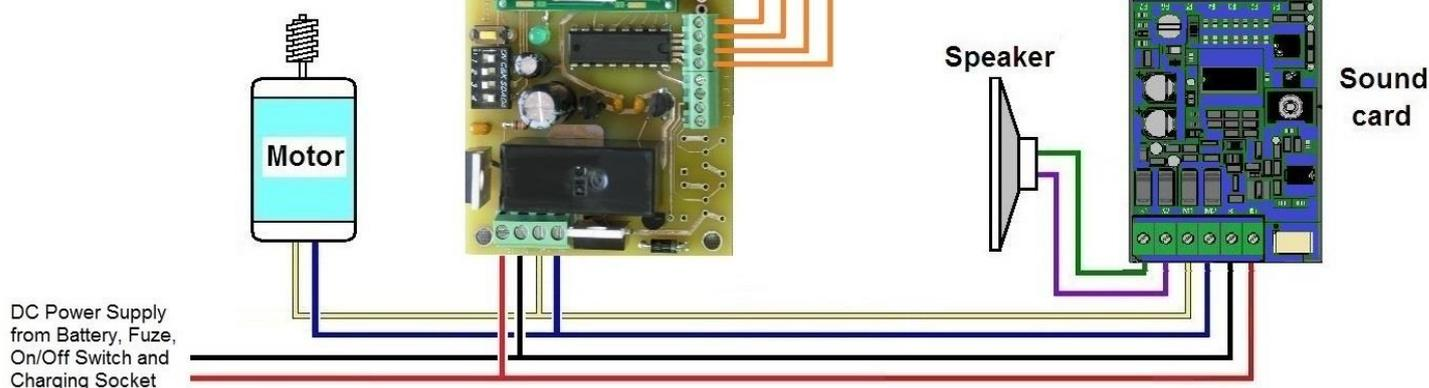
The RailBoss 4 can trigger four sound functions. The fifth and sixth soundcard triggers, the turbocharger and engine start/stop, therefore cannot be radio controlled and will need to be switched on, if required, by the IR remote control or be set to sound automatically. .
