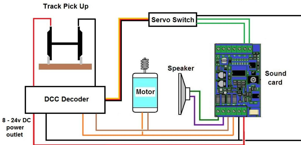
can be used to trigger sounds from the controller buttons by using a servo switch. They may also have a constant DC power output which can replace the battery if it is in the voltage range 8 to 24 volts. These connection options are shown below:
