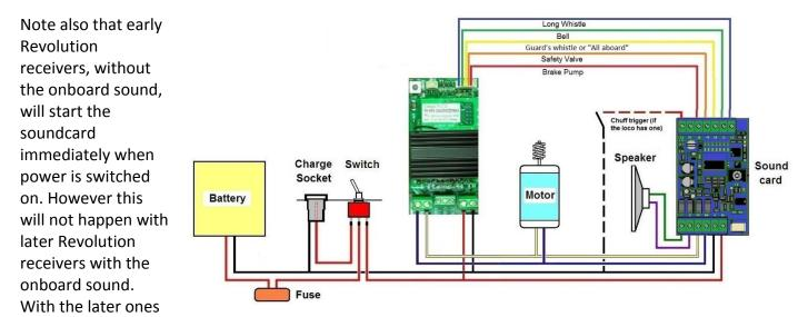
you will need to throttle up three button presses to switch on the sound which will then stay on.
