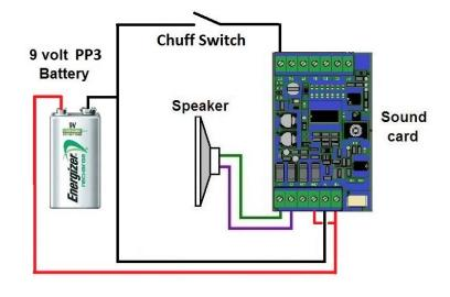
The most common way of doing a chuff switch is to use a reed switch positioned close to the back of a tender or van wheel and then glue magnets around the back of the wheel as follows:
