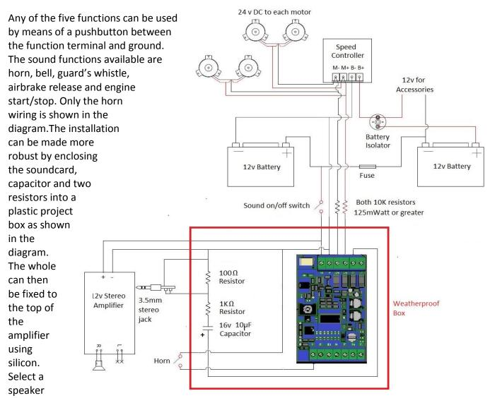
which matches the impedance and power output of the amplifier. In the case of the Jaycar AA0487 a 15 watt speaker of four ohms impedance is needed. It is also important to make a soundbox which is an airtight fit to the back of the speaker. This will improve both volume and sound quality.
