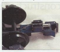
so that it pops open, and the "trip pin" is a metal rod connected to the electronic solenoid. When the solenoid is energized, it pulls this rod back, thus releasing the knuckle.
