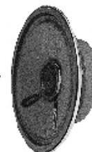
The lowest cost option is to fit a speaker from your local consumer electronics store. Typically these come in 27mm or 57mm diameters. Use the largest which you can fit in your loco.
