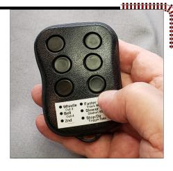
The spec for the radio component used in the RailBoss 4 is 0.5 miles (2,640 feet) outdoor line of sight! We could use that spec, and you would really be impressed. But we know that isn't going to happen in the real world of garden railroading.
