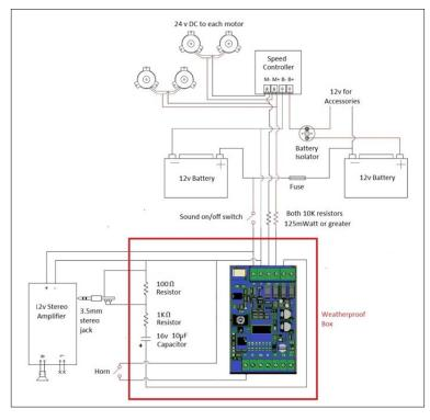
Any of the five functions can be used by means of a pushbutton between the function terminal and ground. The sound functions available are horn, bell, "All aboard", airbrake release and engine start/stop. Only the horn wiring is shown in the diagram. The installation can be made more robust by enclosing the soundcard, capacitor and two resistors into a plastic project box as shown in the diagram.
