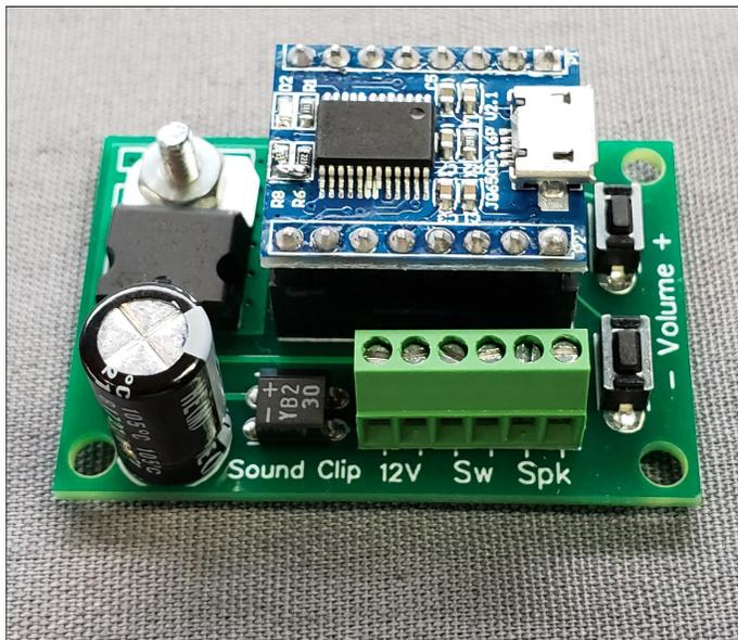
A momentary switch closure will trigger the sound track to play once. Switch can be mechanical or an open collector output from other electronics to the left side of "Sw", and common to the right side of "Sw".
