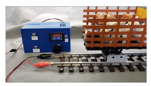
The track output has a connector so different connection options can used. The battery pack can be charged from the front panel, but the snap-lid box and battery connector makes changing out the battery quick and easy if needed.
