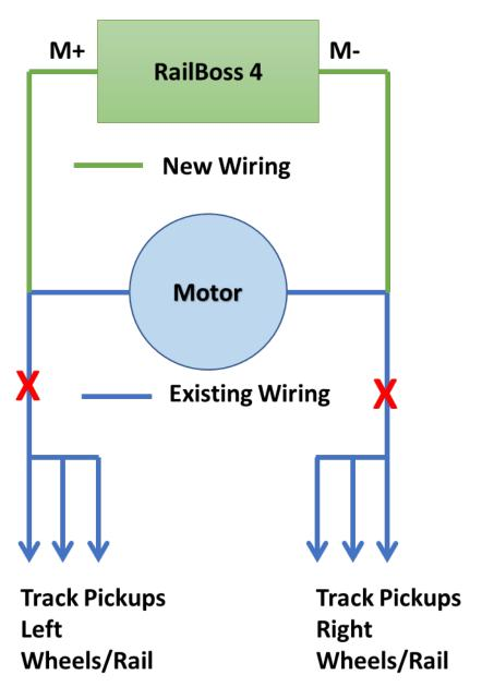
loco that also hasn't disconnected its track pickups will put also put power to the track.
