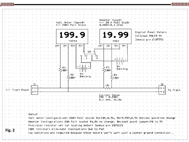
displays. The LCD displays use much less current making it the choice for a stand-alone 9 volt battery powered unit. The LED displays are much easier to read, but will drain the battery faster.
