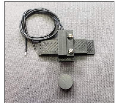
Hardwired Track Reed Switch (to SS, COM) and Loco Magnet
